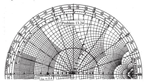
On the chart, radial lines are drawn at positions corresponding to  $.025\lambda$  increments on the WTG scale. The intersections of the lines and the circle give a total of  $11~z_{in}$  values. To these we add normalized impedance of 40/50=0.8 to add the effect of the  $40\Omega$  resistors and obtain the normalized impedance at the line input. The magnitudes of these values are then found, and the results are multiplied by  $50\Omega$ . The table below summarizes the results.
