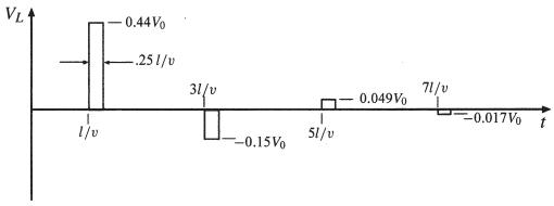
13.40. In the charged line of Fig. 13.22, the characteristic impedance is  $Z_0 = 100\Omega$ , and  $R_g = 300\Omega$ . The line is charged to initial voltage  $V_0 = 160$  V, and the switch is closed at t = 0. Determine and plot the voltage and current through the resistor for time 0 < t < 8l/v (four round trips). This problem accompanies Example 13.6 as the other special case of the basic charged line problem, in which now  $R_g > Z_0$ . On closing the switch, the initial voltage wave is
